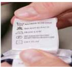
HL35 is a versatile resin that can be used on both textile labels and in traditional TTR applications. It provides good resistance to heat, scratching, and chemicals. It is ideally suited to printing on Cetus<sup>®</sup> textile labels and will withstand washing, ironing, and some dry cleaning.
